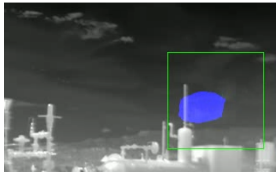
Fig. 4: Processed footage of a correct detect. Distance: 18.6m, emission rate: 109.5 \pm 2.5 scf/hr ( 1806.1 \pm 41.4 g/hr)
